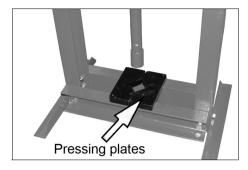
and MUST be of sufficient size with sufficient surface area, so as to avoid the possibility of slipping or springing out. Mating surfaces MUST be horizontal so that the force being exerted will NOT be at an angle.
